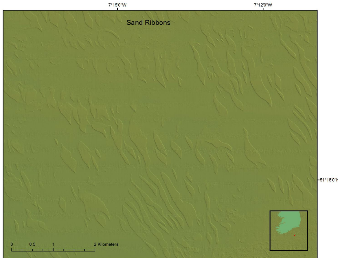
Figure 22: Multibeam shaded relief image showing sand ribbons.
