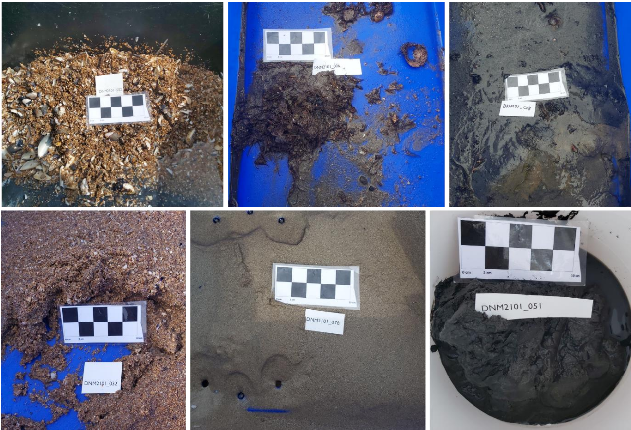
Figure 5. Sediment images from six locations sampled during the current survey. The images show the variability of substrate types in Achill Bay including (from top left) Very coarse sand with biogenic material; Very fine sand mixed with biological detritus; Very fine silt; Coarse sand of variable grain size; Fine well-sorted sand; Thick silt/clay.
