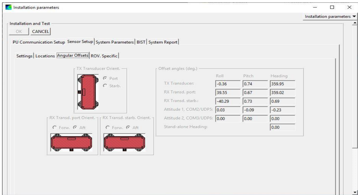
Figure 6: Angular offsets in SIS prior to patch test.
