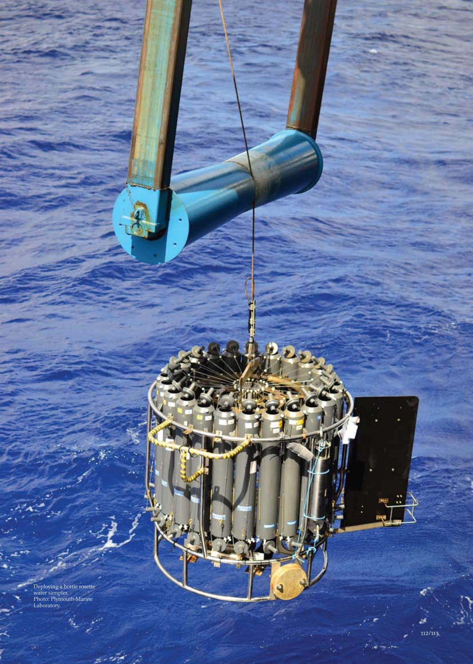
Deploying a bottle rosette water sampler.
