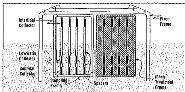
Figure 2. Schematic diagram of the sampling apparatus used in the study. For the 3- and 6-mm treatments, mesh bags were slipped over the sample frame.
